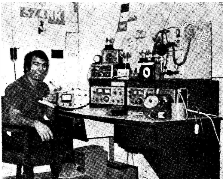
Station of D. G. Simmons, 5Z4NR, Kenya, now G4AVB, 37 Berry Road, Stafford. Gear shown here includes FT-400 Tx, FR-SDX400 receiver with various home-built ancillaries and a two-metre 50w. Tx. Aerials out there were a TA-33Jr. rotatable, a "G5RV" type and a dipole cut for 40m. While in Kenya G4AVB/5Z4NR was one of the radio-link stations for the famous East African Safari Rally.
